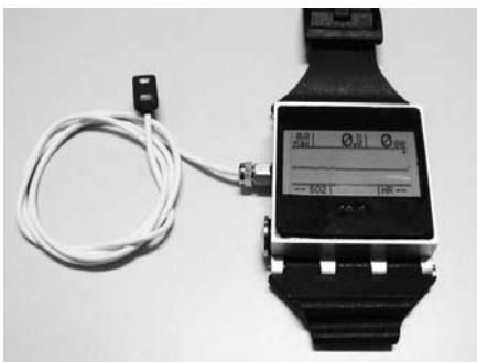
The prototype wrist mounted apnea diving computer
